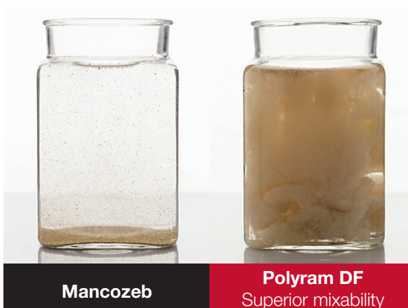
Comparative dispersion of 4 g in 2 L of water 20 seconds after addition without agitation.
